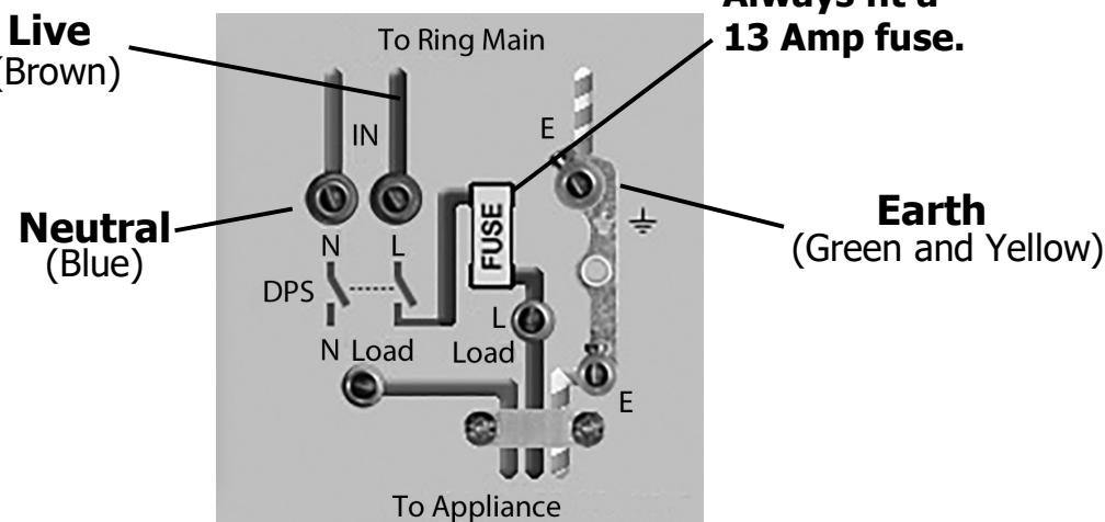
**Ensure that the outer sheath of the cable is firmly held by the clamp**
